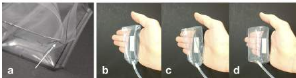
Figure 6. Box prop folding structure illustration. a) Top surface of the material is folded inward before heat-sealed. b) Deflated state. c) During inflation. d) Fully inflated.
